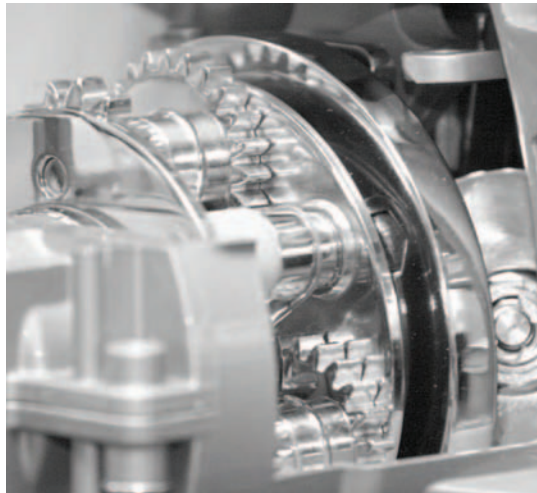
The full toroidal variator transmission: set to tackle conventional gearboxes?
